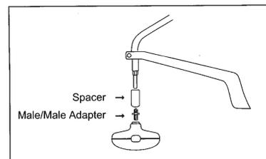
Remove head bolt counterclockwise. Remove entire head, including upper housing. Slip spacer onto shaft as shown. Screw male/male adapter into arbor shaft and No-Brainer™ quick loader head is ready to use.
