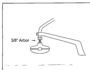
After removing original head (unscrew counterclockwise), replace with No-Brainer™ quick load head. Ready to use.
